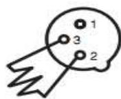
Termination reduces signal errors and avoids signal transmission problems and interference. It is always advisable to connect a DMX terminal, (Resistance 120 Ohm 1/4 W) between PIN 2 (DMX-) and PIN 3 (DMX +) of the last fixture.
