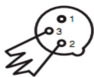
Termination reduces signal errors and avoids signal transmission problems and interference. It is always advisable to connect a DMX terminal, (Resistance  $120\text{ Ohm } 1/4\text{ W}$ ) between PIN 2 (DMX-) and PIN 3 (DMX +) of the last fixture.
